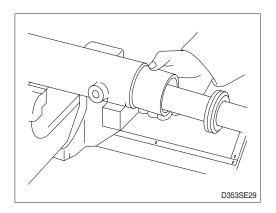
(5) Using a hook spanner, install the gland assembly, and tighten it with torque  $40\pm4$ kgf  $\cdot$  m (289 $\pm2$ 9lbf  $\cdot$  ft).
